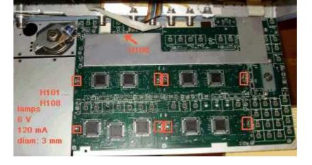
**No monitor speaker audio?** Replace H100 lamp on the front panel just besides INPUT 2. This lamp is inside a black heat shrinking tube (it does not light up anything, so is it as hour counter for service?). Exact value is so far unknown, but audio works and the 24 V 20 mA lamp glows very faintly - find out the proper voltage and current, or use what lamp you have - at your own risk!
